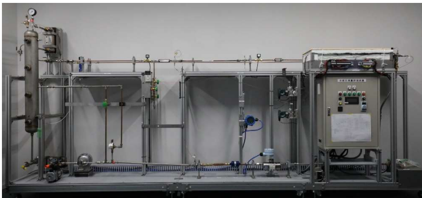
Heat transfer & void fraction measurement system
